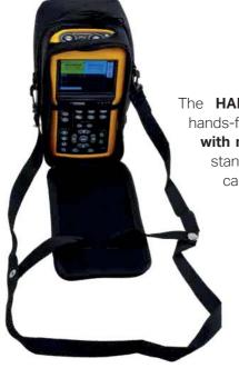
The **HANDSCOPE's** essential feature, hands-free use, is facilitated by the **bag** with **neck-strap** and the magnetized stand supplied for fastening on metal cabinets.
